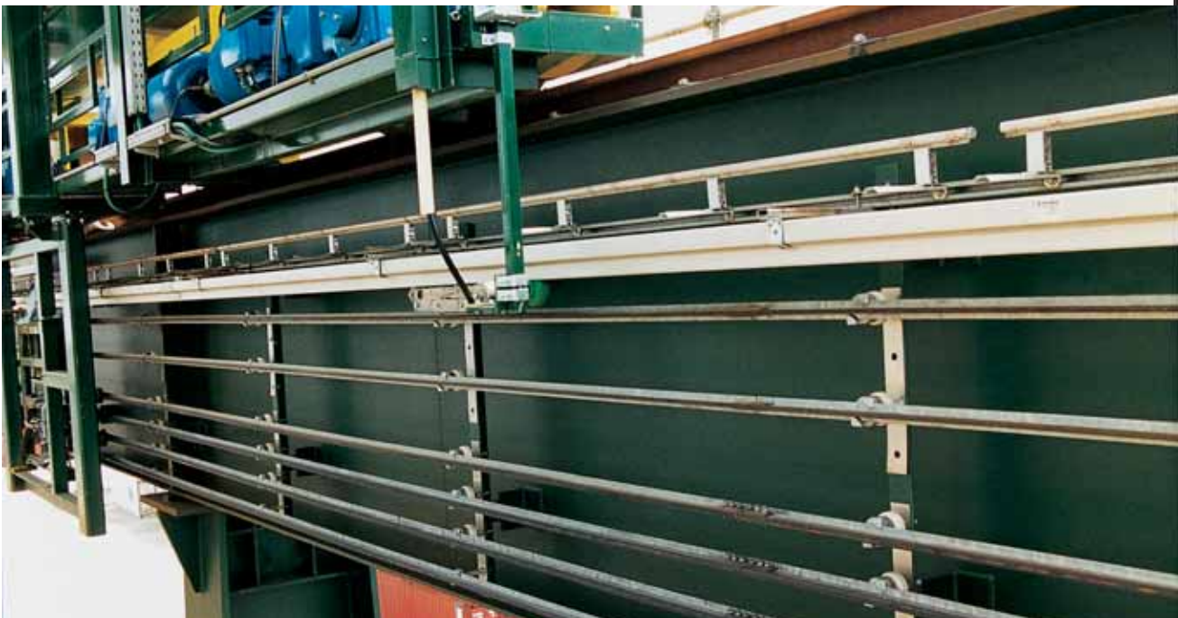
Antenna guiding SMG-RAE-XY-6 in use at a large crane application.
