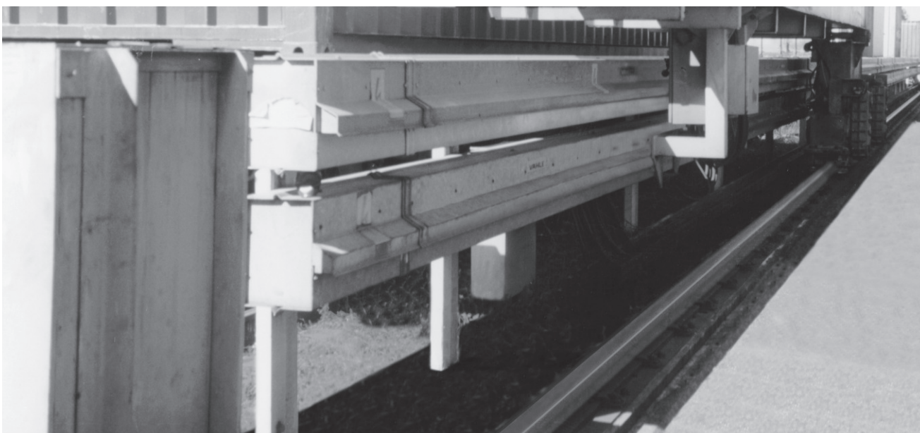
VAHLE FK-system for container terminal
