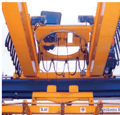
Supply of the turning-cab on an EOT-crane
